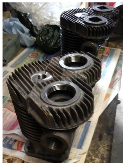
Above picture shows a machined barrel alongside a non-machined barrel. Bottom pictures show a view of the bore of both the above barrels.
